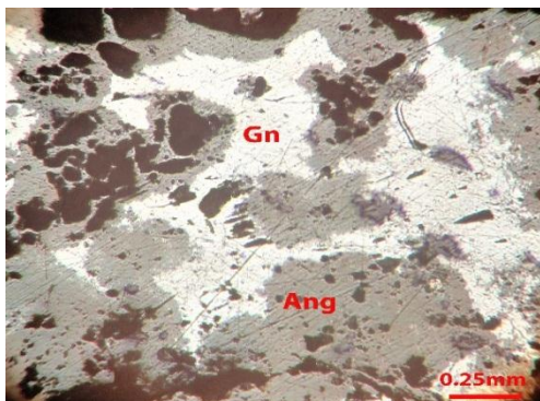
Figure 35 Galena is replaced and rimmed by intergrown anglesite (Gn = Galena, Ang = Anglesite) (Polished Section)
