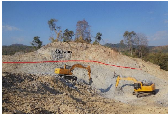
Figure 16 A Gossan capping the Taung Gaung orebody (Location: 96°20'2.0" E and 22° 7' 27.982" N) Facing: East
